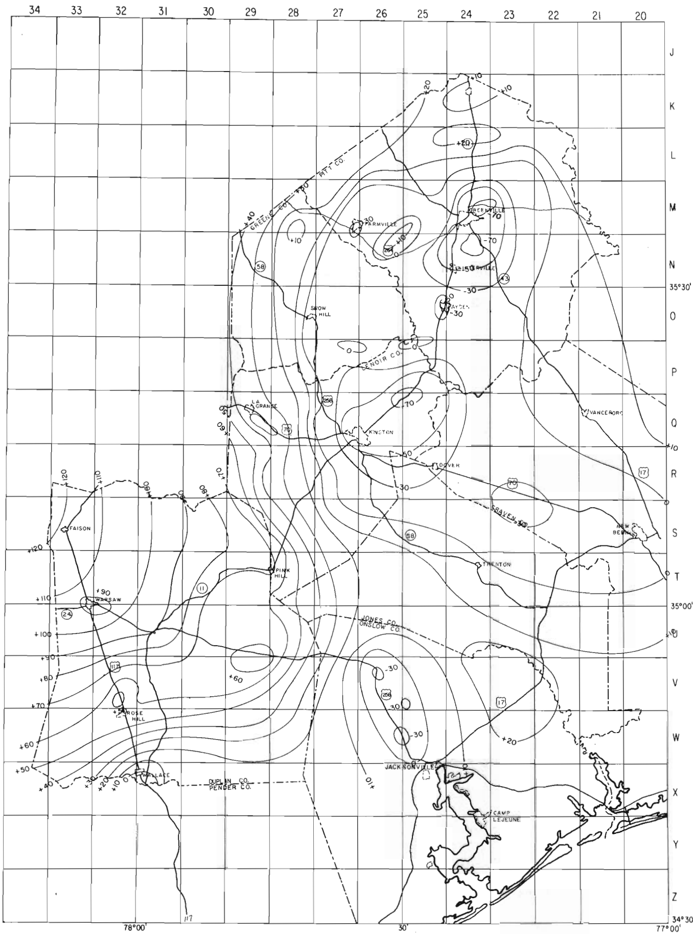
FIGURE 37—ELEVATION OF THE POTENTIOMETRIC SURFACE IN THE CRETACEOUS LOWER SAND UNIT IN 1979
