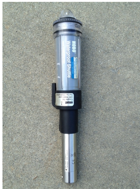
Electronic water level recorder (Hobo connected to Shuttle)
