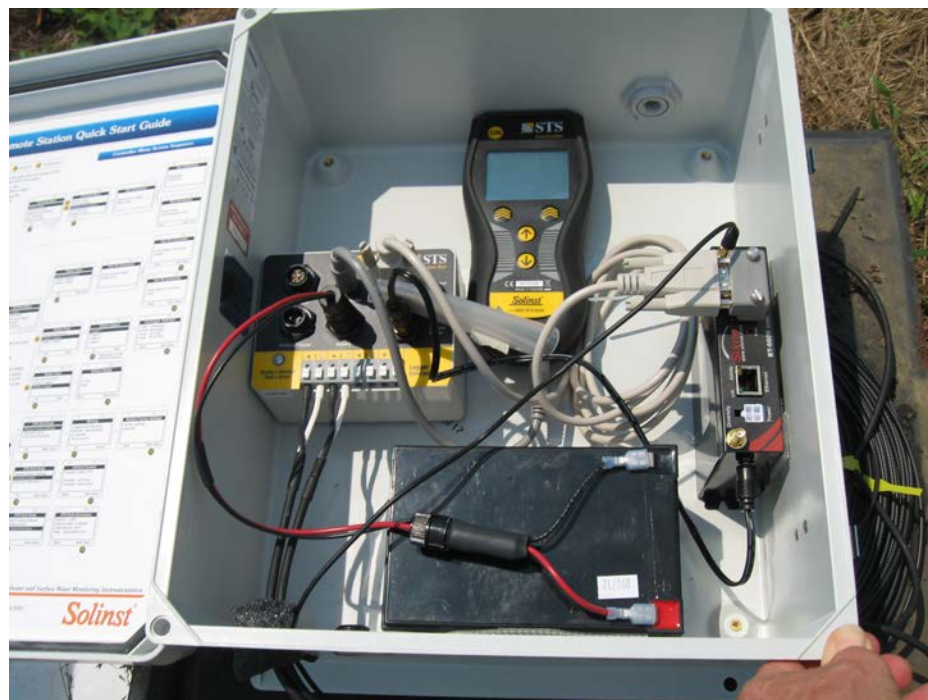
Solinst Telemetry System
