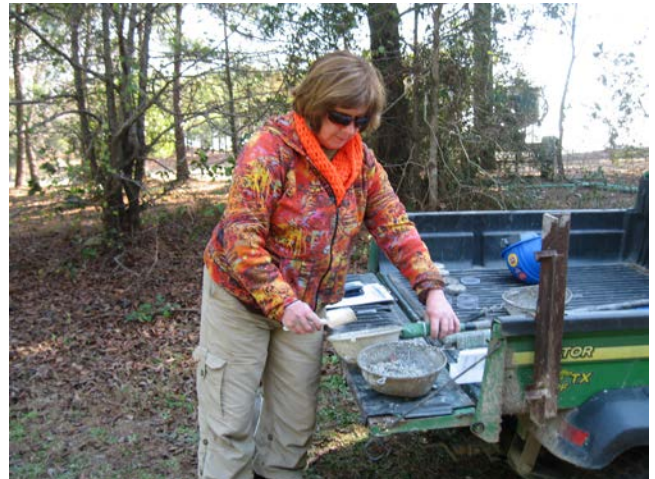
Collecting drill cuttings for lithologic interpretation
