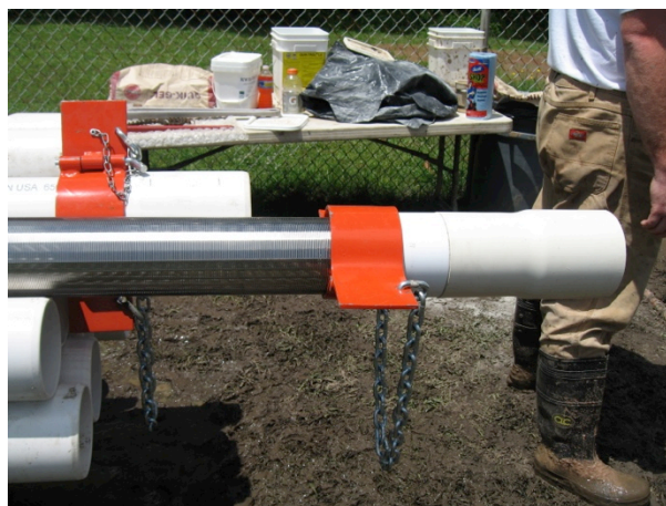
Slotted Screen with Tail Pipe
