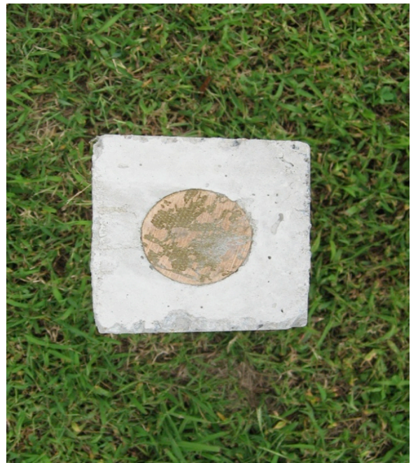
Top of monument - survey point
