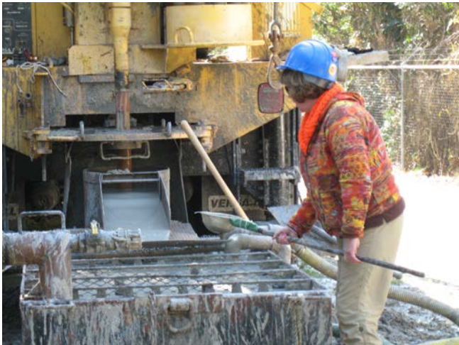
Collecting drill cuttings for lithologic interpretation
