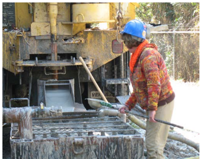
Collecting drill cuttings for lithologic interpretation
