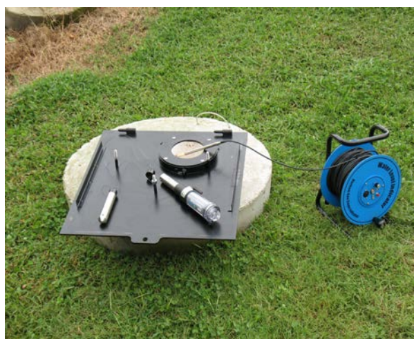
Hobo Including barometer, shuttle, and water level indicator
