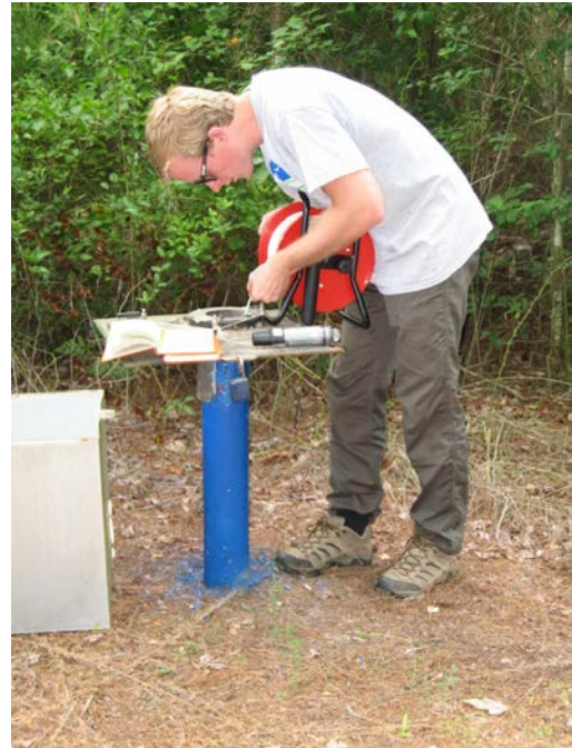
Manual Water Level Collection
