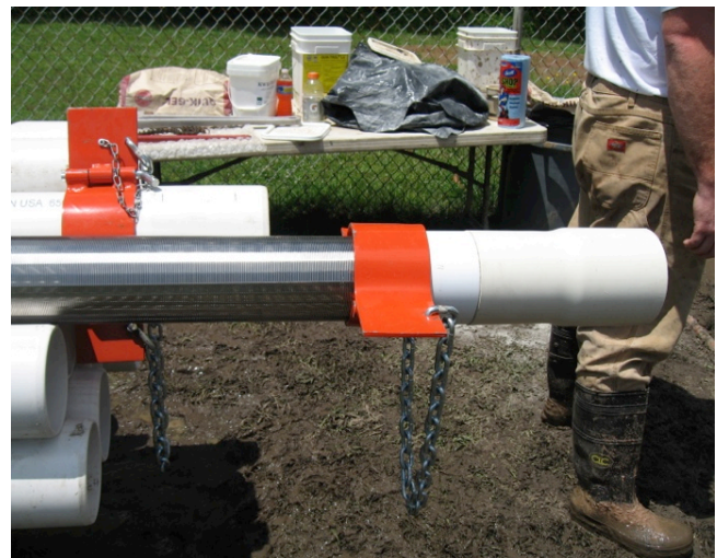
Stainless Steel Slotted Screen with Tail Pipe
