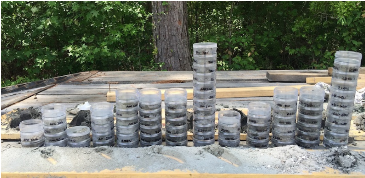
Samples Collected from Drill Cuttings Holly Shelter Station, Z29N, Pender County
