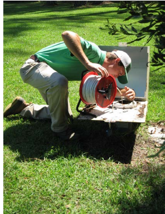
Manual Water Level Collection Comfort Station, U26J Jones County
