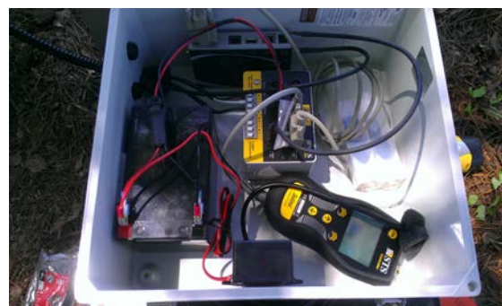
Solinst Telemetry System (STS) Rowland Station, Z 47R, Robeson
