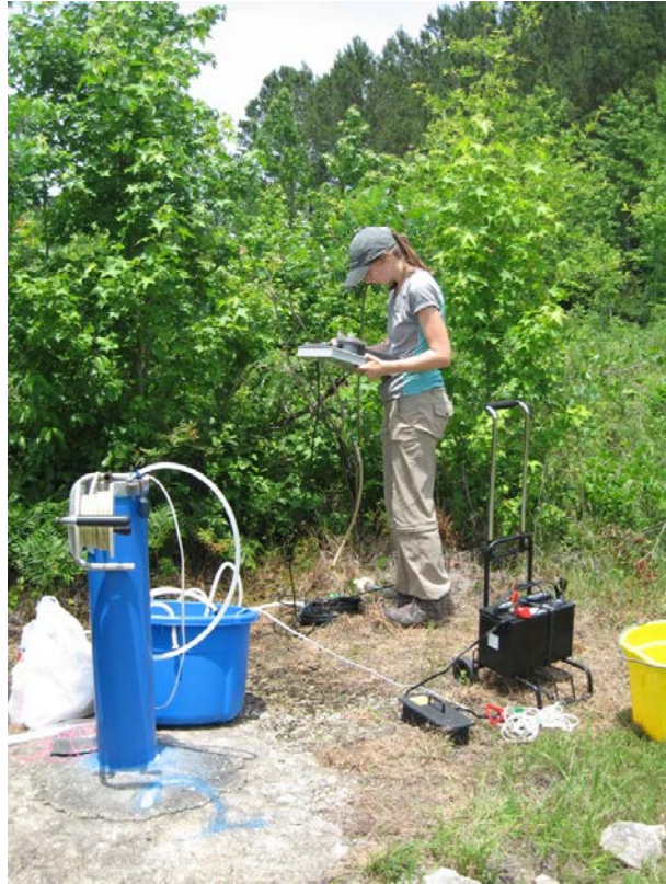
Purging Well Prior to Sample Collection Western Research Campus, M 25F Pitt County
