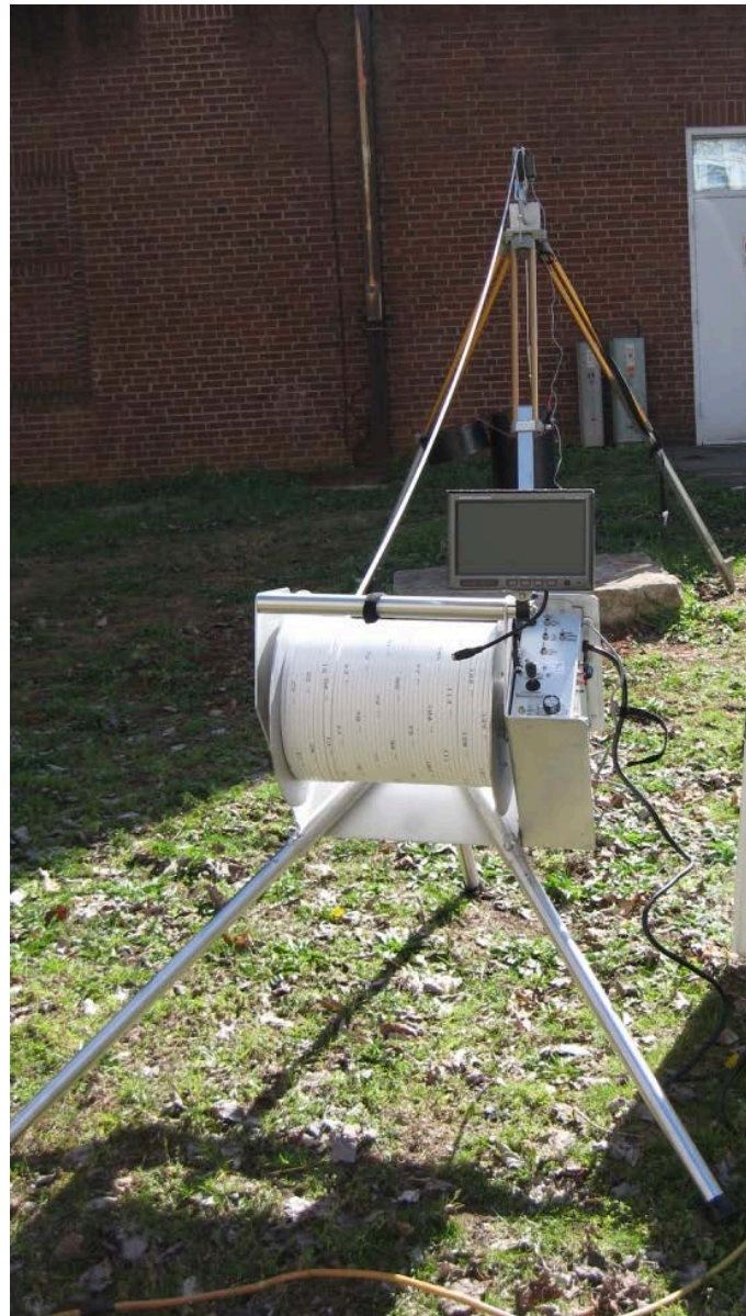
Down Hole Camera (Video-Logger) Stillwell Building, Q 94J, Jackson County
