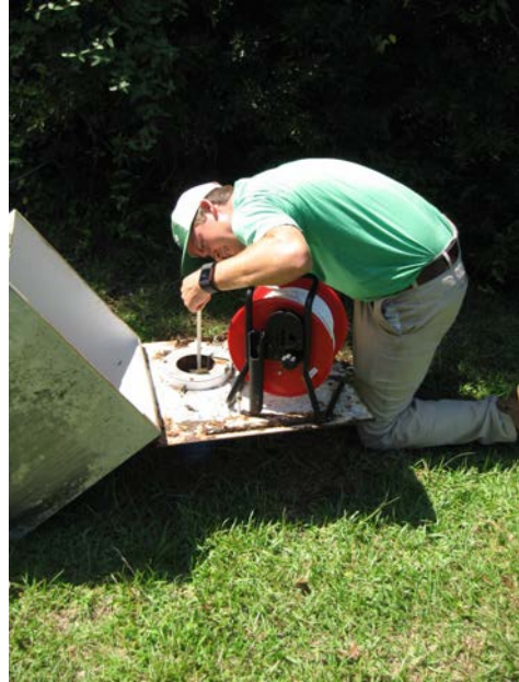
Depth to Water Level Measurement Comfort Station, U 26J, Jones County
