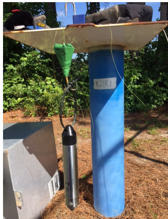
Hobo Datalogger Bear Grass Station, K 21R Martin County
