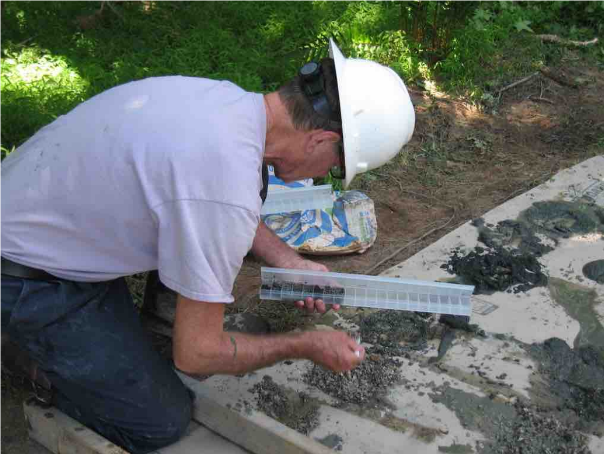
Collecting Samples from Drill Cuttings, Merchants Millpond Station, C 16S, Gates County
