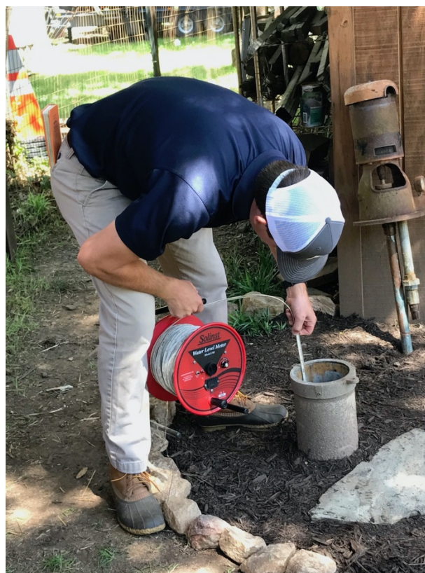
Depth to Groundwater Measurement Powell Drive (K 40M) Raleigh, Wake County, NC
