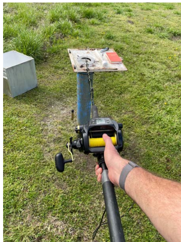
Chloride Sampling Deppe Monitoring Station, V23X Onslow County, NC
