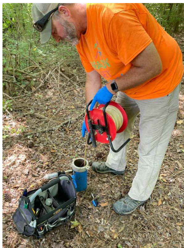
Depth to Water Measurement Godley Monitoring Station, Q16G Beaufort County, NC
