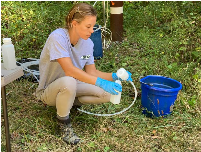
Groundwater Sampling for Metals Using 0.45 \mu m Filter Bent Creek Station, O87D Buncombe County, NC
