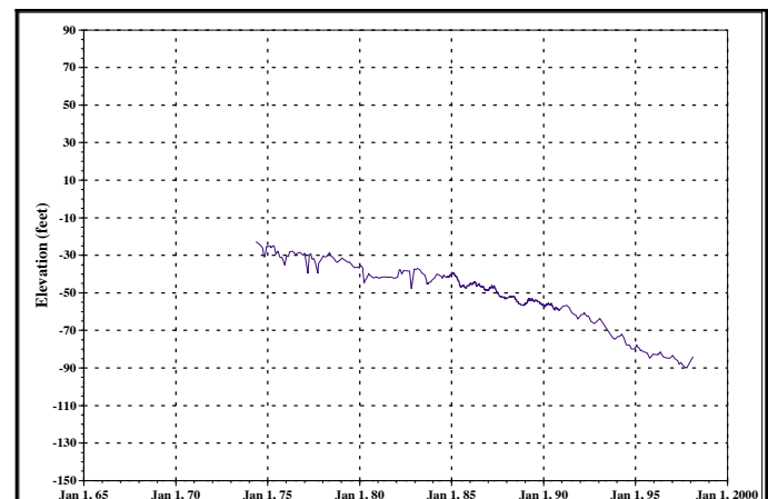
Figure 5. Hydrograph of Upper Cape Fear aquifer well near Kinston, NC.
