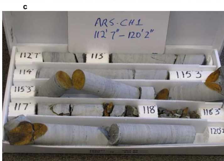
Figure 6. Core photographs showing (a) disc-shaped pyrites on a horizontal fracture, (b) pyritic crusts on subvertical and horizontal fractures, and (c) a fractured section (113' – 120') showing evidence of water-rock interactions.
