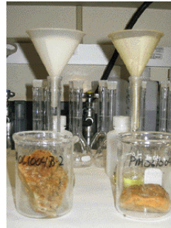
Nitric – hydrochloride extraction on heat plate
