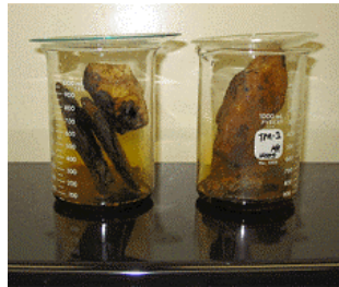
Nitric – hydrochloride extraction on heat plate
