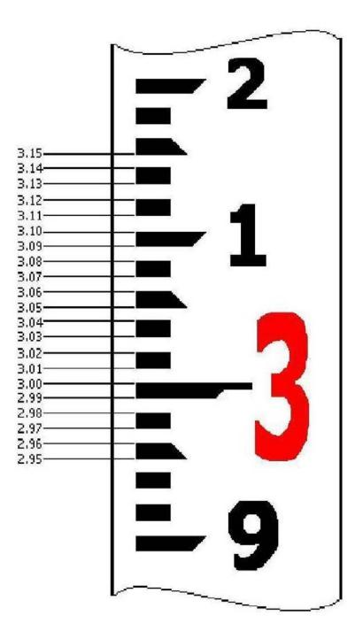
Figure 1. Diagram of a portion of a typical leveling rod showing how to read graduation marks. Each black bar and each white space between the bars is equal to 0.01 feet thick.
