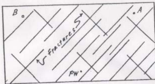
Figure 8.26. - Differences in response of observation wells caused by aquifer anisotropy.
