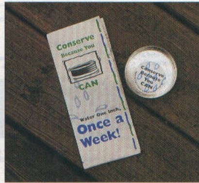
The town used "The Tuna Can Plan" to help residents lower irrigation levels of lawns and gardens. Steel cans 1 in. (25 mm) deep were distributed, and residents placed them under sprinklers—helping them judge when 1 in. (25 mm) of water had been applied.
